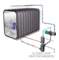
Closed loop cascade jacket cooling system recycles steam condensate, cooling it through a closed loop heat exchanger and recirculating it over the chamber to assist in cool down during liquid loads.
