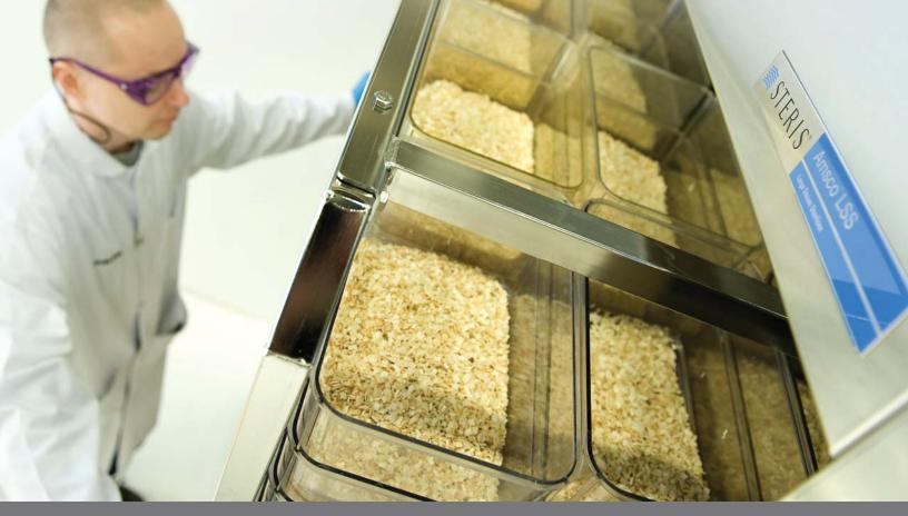
The AMSCO LSS Sterilizer is designed to process laboratory animal caging systems and associated equipment. The LSS incorporates several features to maximize productivity, provide flexibility, and ensure safety and reliability. The LSS was also developed with the sustainable laboratory in mind.
